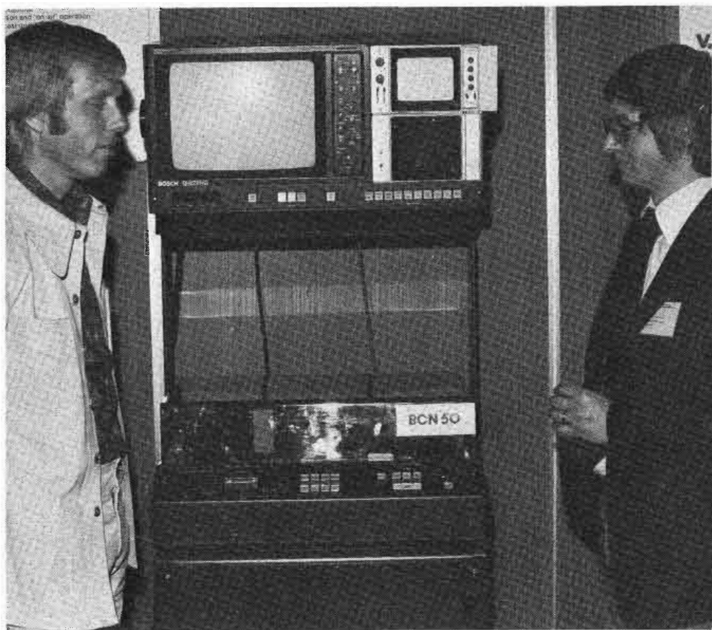
Bosch/Fernseh exhibit at Montreux included VTR's in different configurations. This studio version includes picture and waveform monitor in an over-console bridge.
